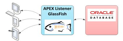
This browser centric user interface (UI) allows APEX to be accessed from any device that supports a browser. This allows an APEX application to be displayed on a PC, Tablet or Smart Phone. APEX automatically identifies the device and then switches to UI conventions that a common on that device. As an example: - iOS has certain conventions for date and time List of Value's
