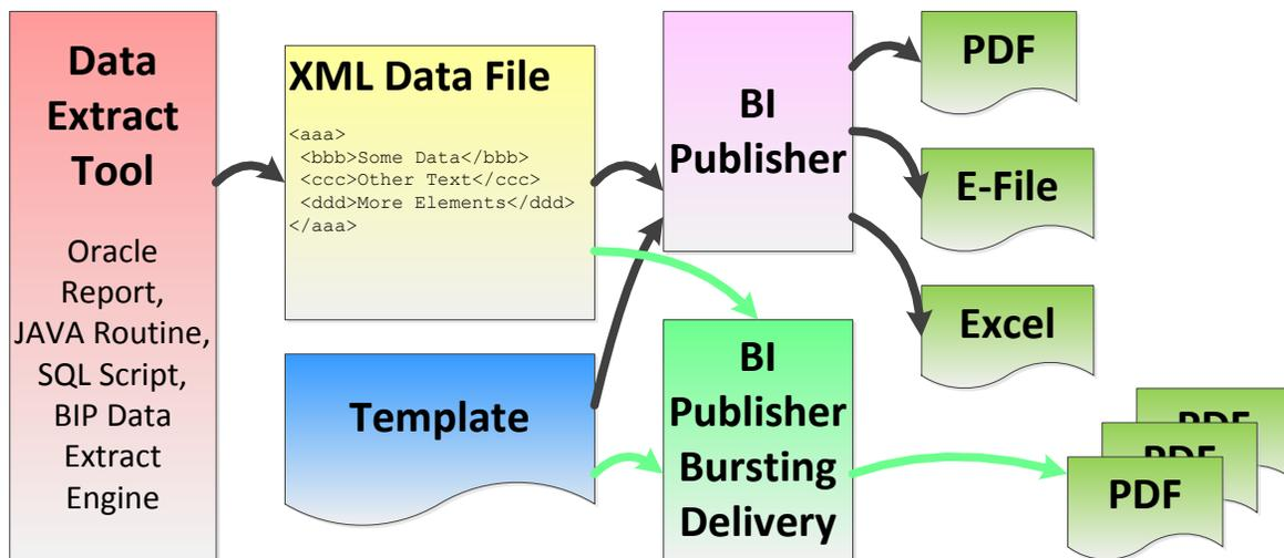
The process begins with the creation of an XML Data Stream using a Data Extract Tool. There are four commonly used tools used to accomplish this:
