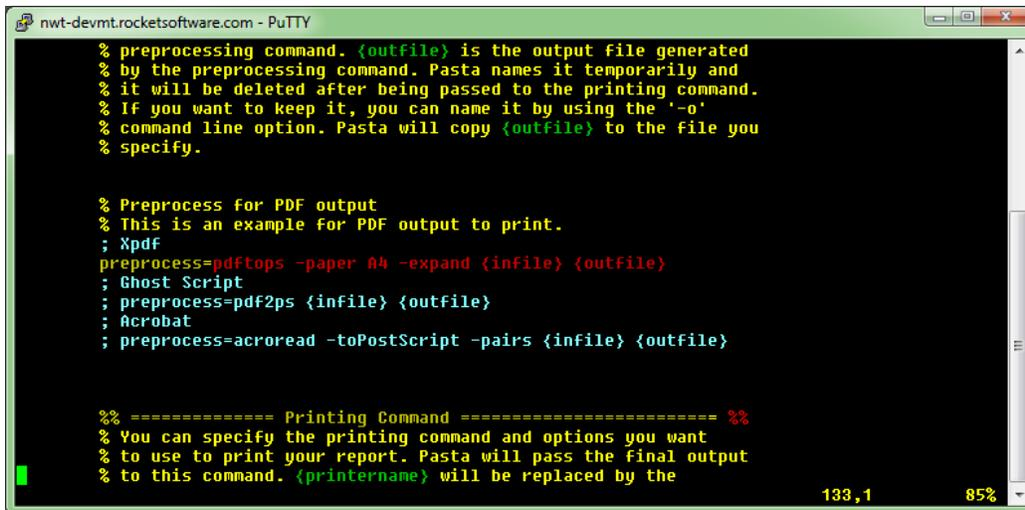
This example uses the conversion utility pdftops (PDF to PostScript). There are equivalents for the other two conversion utilities.
